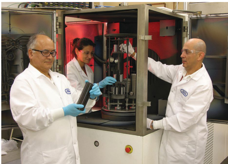
Typical magnetron sputtering system used for the deposition of tribological coatings. (Image courtesy of Argonne National Laboratory.)
